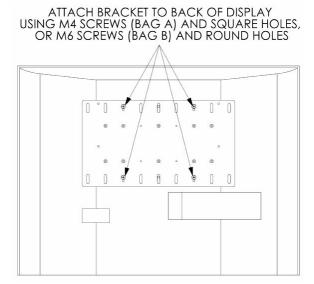
Figure 9. Display with 200mm x 200mm Hole Pattern
